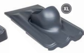
XL Universal MK1 • profiled steel roofing with wave distance 183.3 mm, wave length 350 mm and wave height 39 mm
